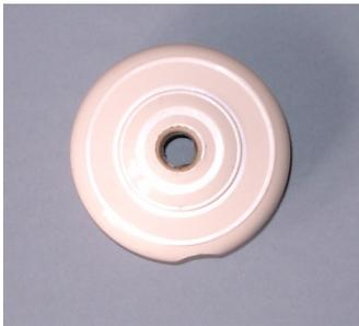
You are not likely to be able to make the precise 12mm. hole that is needed to suit the pipe. My new 12mm. drill produced a hole about 0.5mm oversize.
